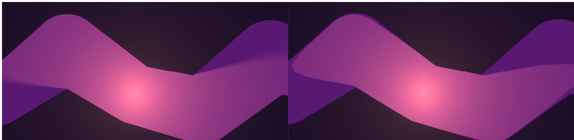
Figure 3 Artifacts from sharp edges (left) and insufficient number of steps (right)
